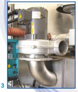
2) DRYING STAGE After the wash and rinse stages, the parts dried with a high velocity (15,000ft/min) blast of hot (typically 260 F) air. For drying, the machine is equipped with a regenerative blower (5 HP for CJ-2, 10 HP for CJ-4), a low watt density air heating system (12.8 kW for CJ-2, 21 kW for CJ-4), and a steam exhaust blower.
