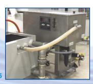
5) OIL SKIMMING For skimming oils from a given tank, there are two options: 1) the OSB-22 motorized belt skimmer. This skimmer has a stainless steel belt and is controlled with a 7 day/ 24 hour timer. 2) the OWC-22 oil water coalescer. This stainless steel coalescing tank is rated for a 1 GPM flow and includes a floating skimmer head and a transfer pump.
